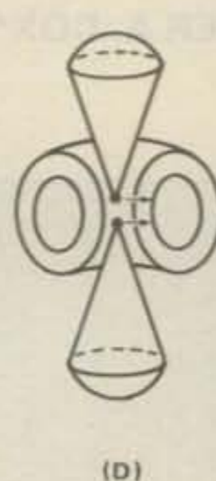
Fig. 4- Evolution of sleeve-dipole antennas from sleeve-monopole antennas.
